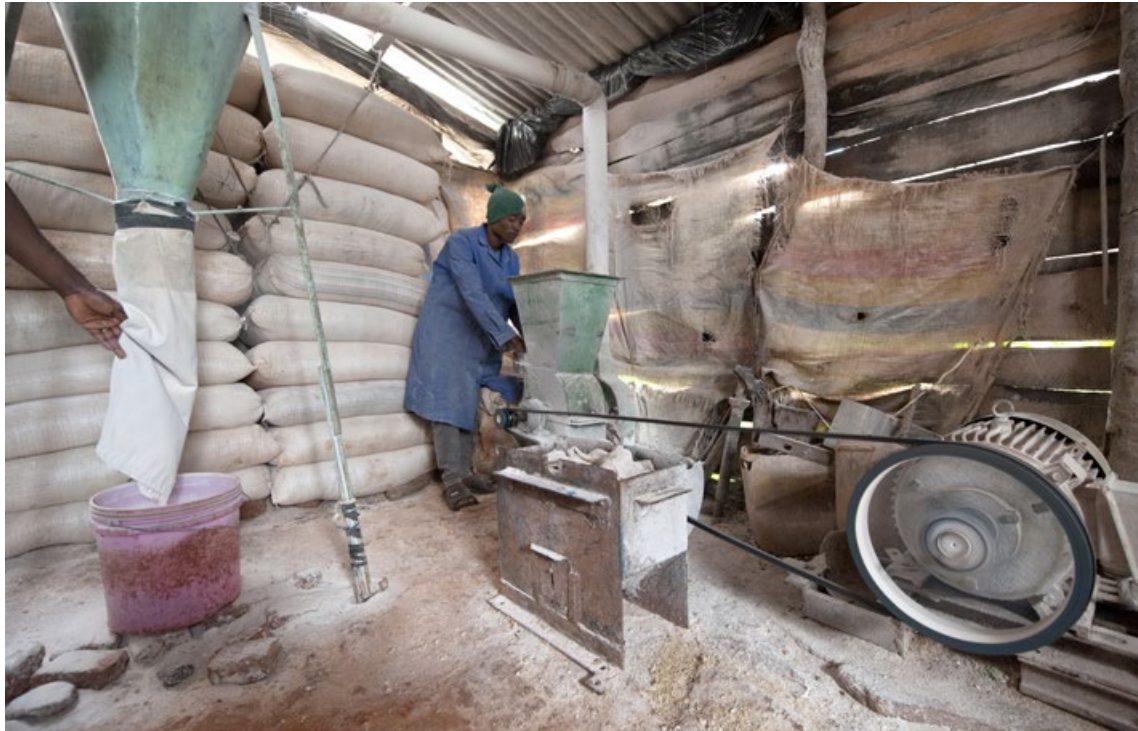
A corn mill in Lichinga operated with electricity from the grid. Electric corn mills can grind corn much quicker and with less effort than a manual grinder. PHOTO: KEN OPPRANN
