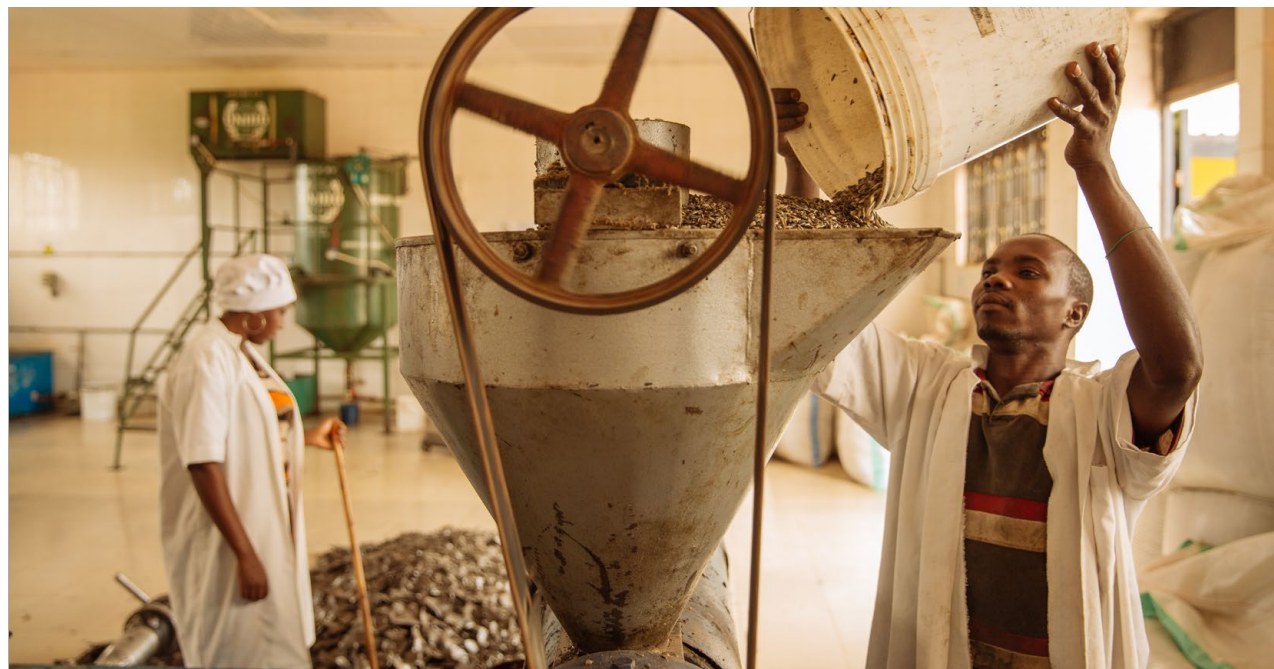
Worker pouring sunflower seeds into an extraction machine in Dodoma, 2016. FOTO: MITCHELL MAHER/INTERNATIONAL FOOD POLICY INSTITUTE
