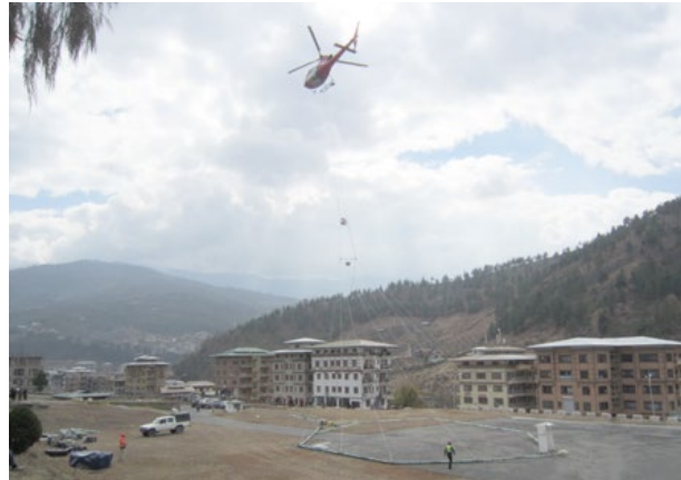
Airborne geophysical survey along Thimphu-Wangdue tunnel PHOTO: NGI
