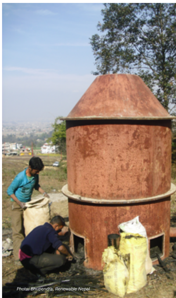
Testing of charring in retorts in Nepal.
