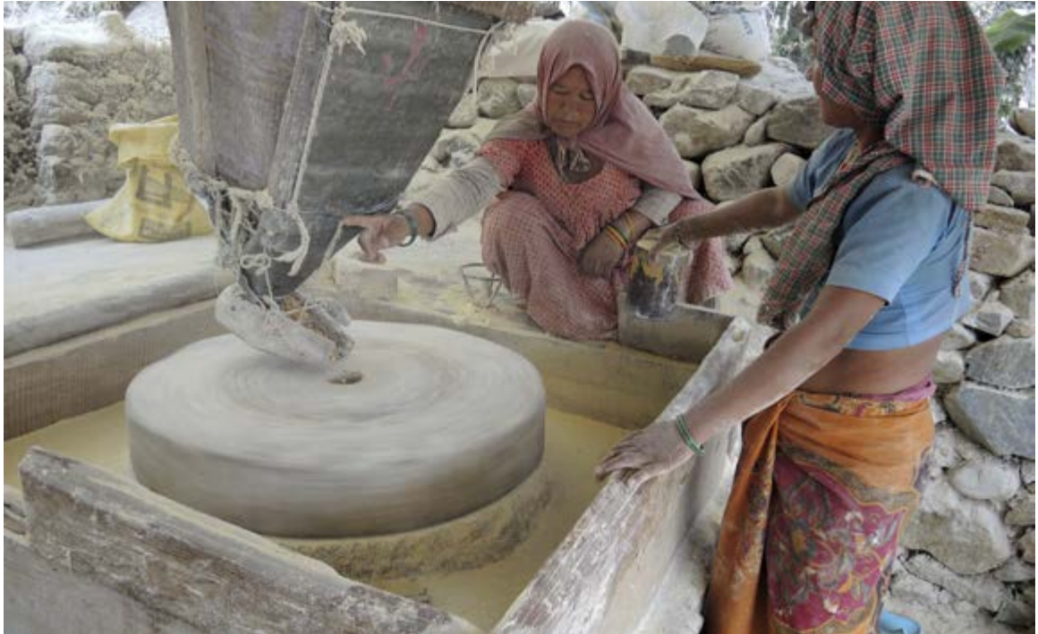
In Nepal, energy services make income-generating work possible for women as well. Here two women are grinding flour using a mill operated by hydropower from a waterfall. This reduces physical work and saves time. PHOTO: ELISABETH CLEMENS
